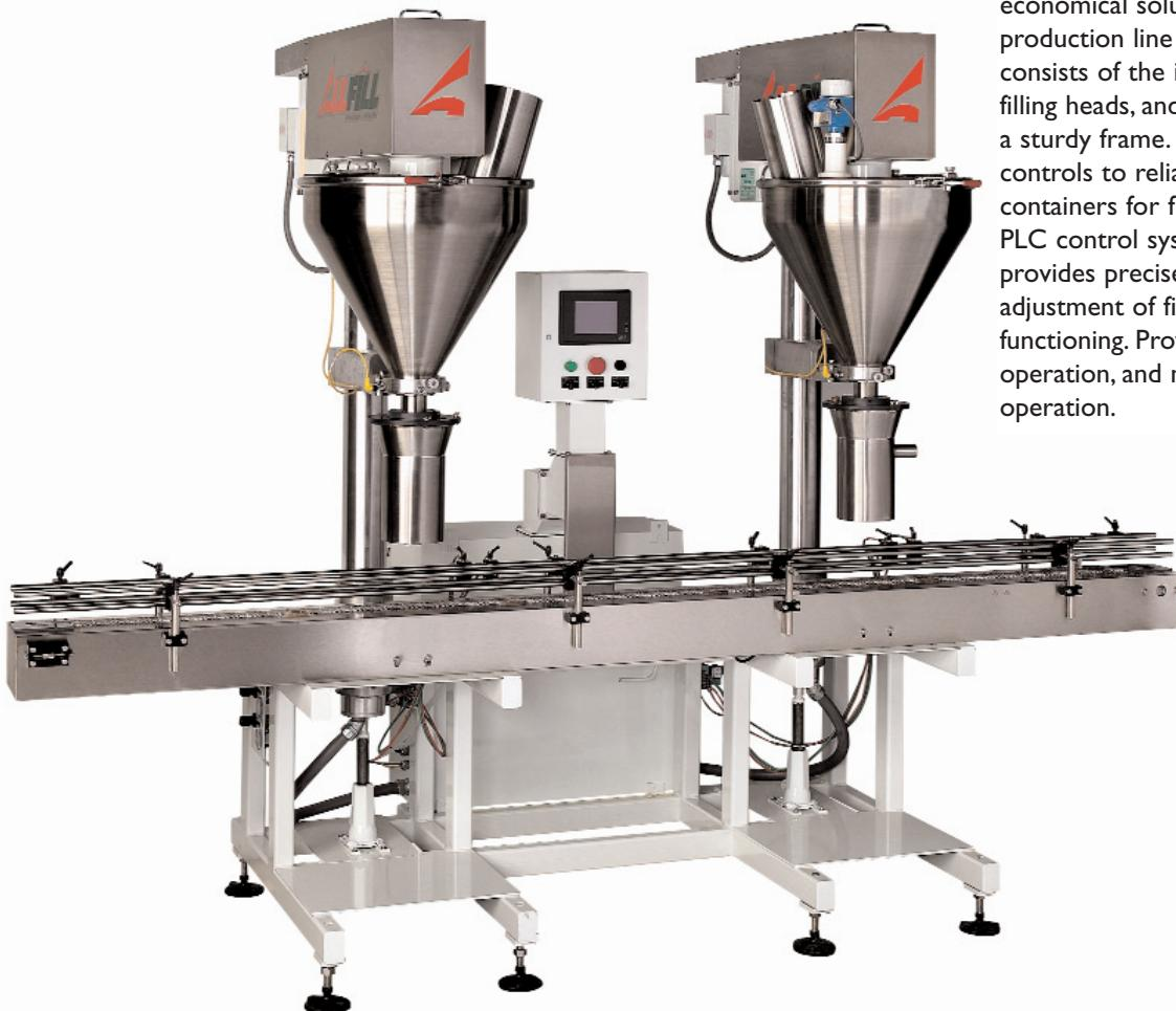
The **Model DHA** is a complete, economical solution to your filling production line requirements. It consists of the industry-proven All-Fill filling heads, and conveyor mounted on a sturdy frame. Container indexing controls to reliably move and position containers for filling. Allen Bradley PLC control system with touchscreen provides precise selection and adjustment of fill amounts and machine functioning. Provides easy setup, operation, and monitoring of the filling operation.
